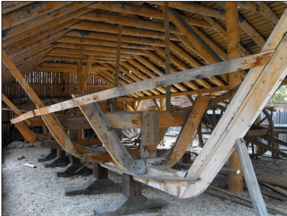
Figure 4-4 Skeleton of York Boat with False Timbers or Moulds in place
