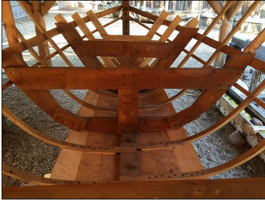
Figure 4-5 Boat Skeleton showing both moulds and real timbers with first planks attached
