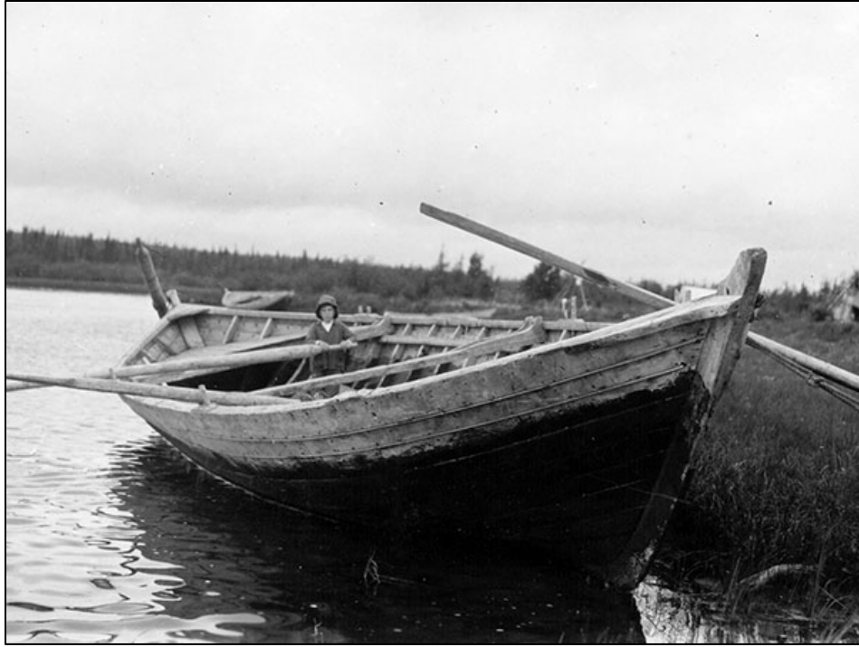
Figure 4-10 York Boat showing Oar Pins, and Platform for Steersman
