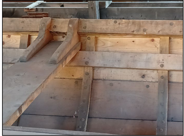
Figure 4-7 Interior of a York Boat showing floor boards, thwarts/thafts, gunwale, and planks attached to timbers
