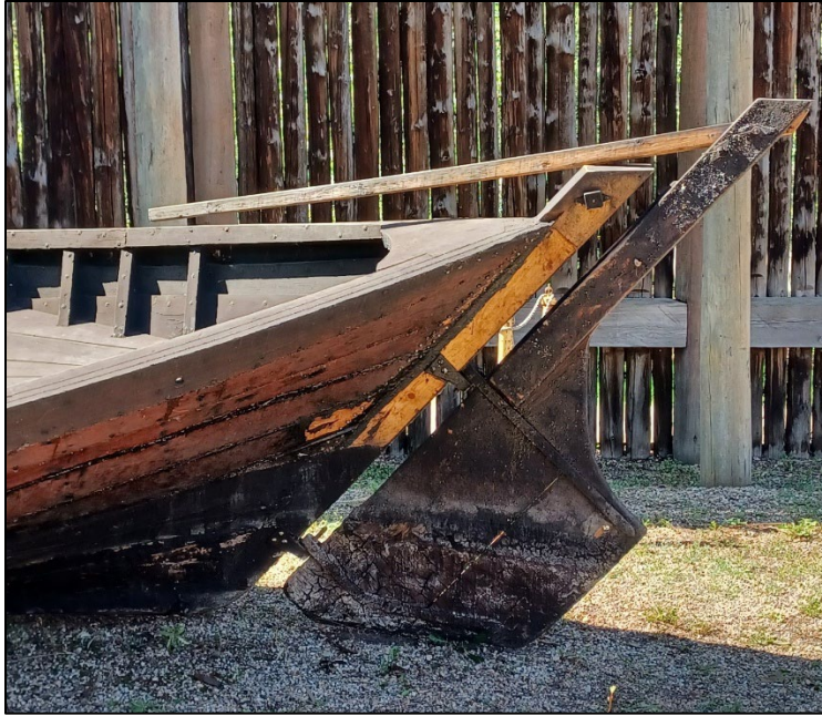
Figure 4-9 Stern of the old York Boat at Fort Edmonton showing the rudder
