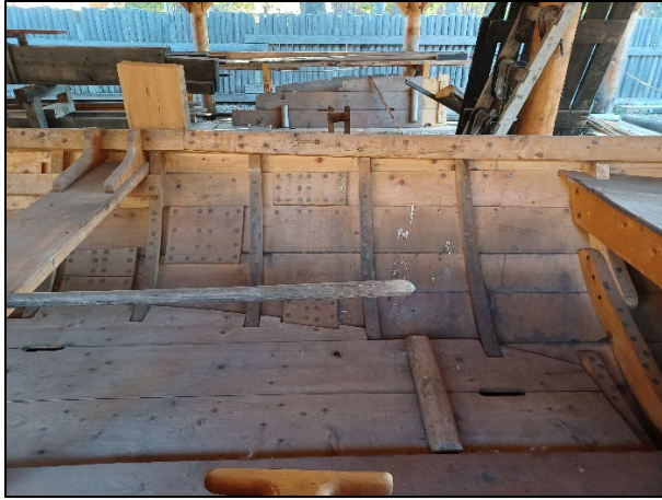
Figure 4-7 Interior of a York Boat showing floor boards, thwarts/thafts, gunwale, and planks attached to timbers
