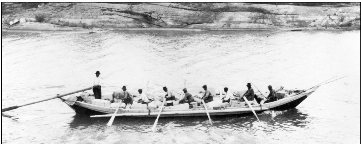
Figure 5-2 York Boat showing alternating rowing positions
